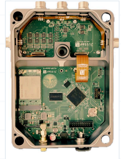
sensor-link hub: main board with LTE modem and a swappable sensor frontend.
