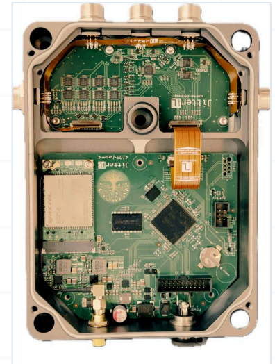
Sensor Link hub: base board with LTE modem and a swappable sensor frontend.
